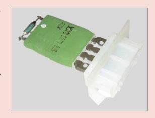
the problem will still not have been rectified. It is therefore only a matter of time before problems recommence and the fuse activates again, meaning the blower will only work at full speed or not at all.
